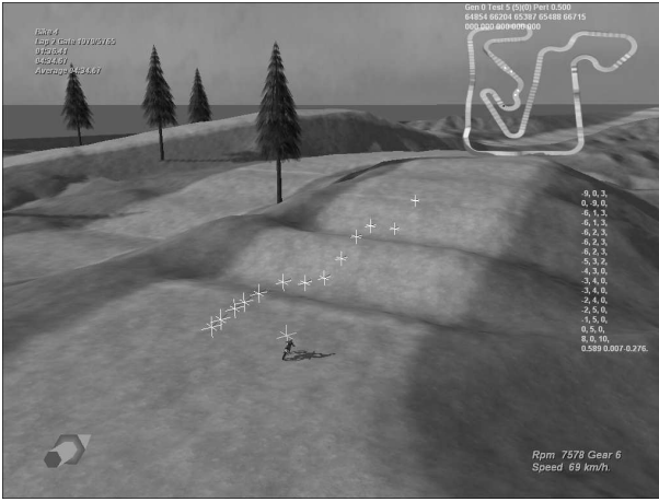
Fig. 1. Screen shot taken from the game; the white crosses represent the position of the track centre lane; there are 13 samples which are used as inputs to the ANN.
