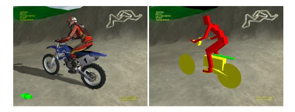
Figure 2.8: Bike Physics: The bike and biker as seen in the game and their associated collision and dynamic objects used in the simulation.
