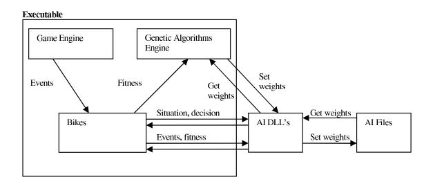
Figure 5.2: Motocross The Force AI SDK Architecture
